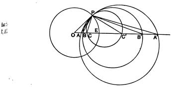
Let E be one of the double points, and let P be any point on the circle whose centre is O and radius OE. The circle which cuts this circle orthogonally and passes through A will pass through A',  $I = \text{ since } OA \cdot OA' = OE^2 = OP^2$ . It is evident therefore that the circles PAA', PBB', PCC' will touch each other at P.
